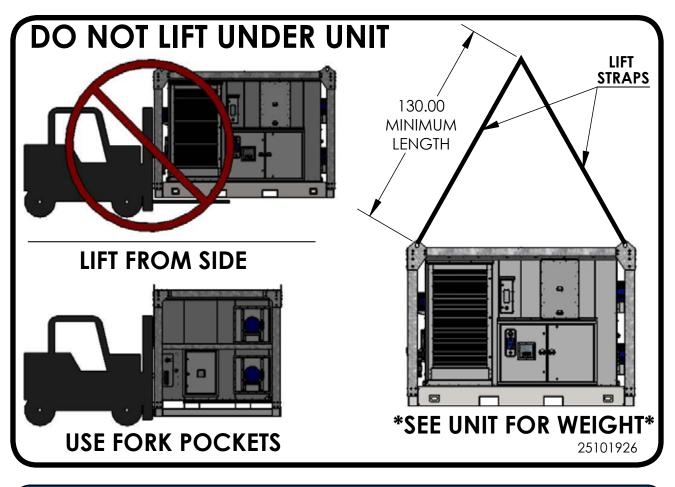
When lifting with a forklift make sure that the forks extend completely through the units lifting holes. Forks which do not reach to the other side the unit could cause it to tip resulting in unsafe conditions or damage to the unit.
