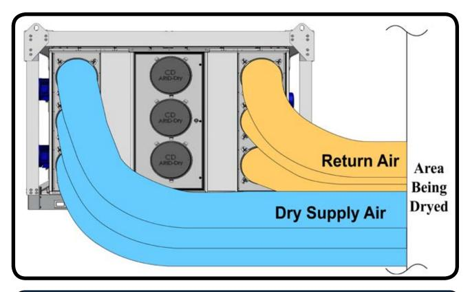
If unit is to be used in a harsh or very dirty environment, it may be better to pull the return air from outdoors rather than pull the contaminated air through the unit. Doing so may damage the rotor.
